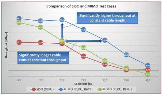
Figure 7 Comparison of SISO and MIMO test cases
