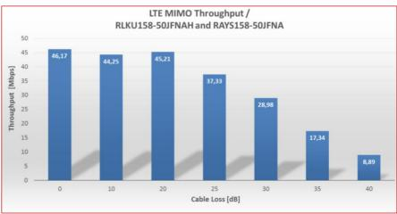
Figure 6 MIMO performance for identical types of radiating cables
