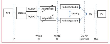
The length of the radiating cable section in the tunnel was 60m. Simulation of longer cable length is done by attenuating the RF feeding power into the radiating cables. The test configuration is illustrated in **Figure 2**.
