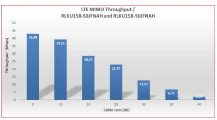
Figure 5 MIMO performance for identical types of radiating cables
