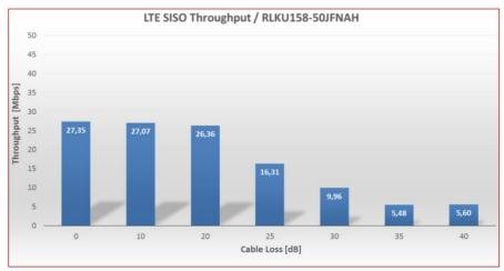
Afterwards, the signal-to-noise ratio degrades with the decreasing RF signal power
