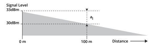
Example: a<sub>l</sub> = 3 dB / 100 m Note: a<sub>l</sub> increases with frequency!
