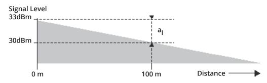
Example: a<sub>l</sub> = 3 dB / 100 m Note: a<sub>l</sub> increases with frequency!
