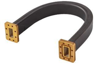
Twistflex is fabricated from spiral wound silver plated bronze strip. Twistflex is provided with EIA or IEC flanges. EIA twistflex includes mounting hardware for one flange. In twistflex with different flange on each end, hardware is supplied for both flanges. IEC twistflex includes gaskets and mounting hardware for both flanges. Standard lengths are 24" (60 cm), 36" (90 cm) and 48" (120 cm).
