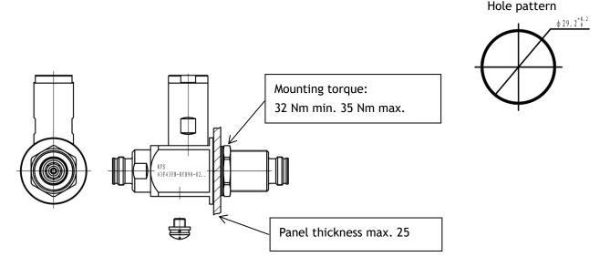
Note: If the grounding of entry panel is not possible, use wire connection as shown under section 2. Sample picture of 43F43FB-HYB90-02. Instruction valid for complete -HYB90-02 series
