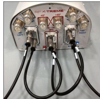
Figure 6 Typical daisy chain configuration
