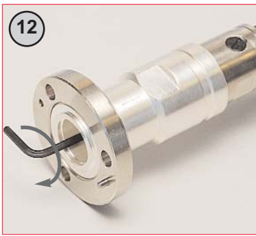
12 Re-tighten inner assembly to a torque of 2.6 Nm.
