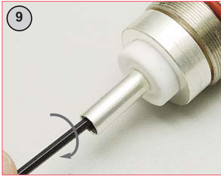
9 Insert inner cable assembly into back nut and finger tighten using M3 hex key.
