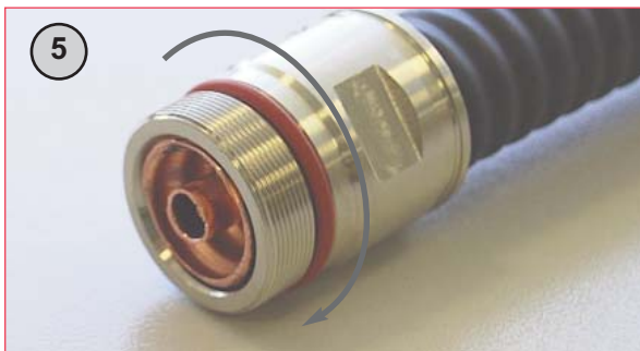
5 Screw back nut clockwise onto the cable.
