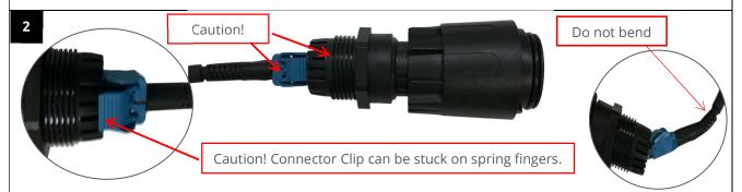
Feed the fiber connector into the sleeve until the Connector comes out. Caution: do not apply too much force as doing so can cause damage to the fiber and gland spring fingers.
