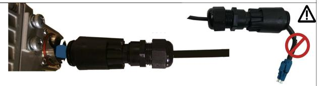
Remove the fiber dust caps from fiber end face and seat into the RRH SPF card slot until you hear a click. Do not twist fiber end face or kink the fiber during installation.
