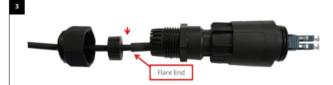
Wrap the rubber split grommet around the jacketing and VERY CAREFULLY push it UNDER the clamping fingers until the grommet is flush with the finger ends. Caution: it will be necessary to gently lift the fingers.
