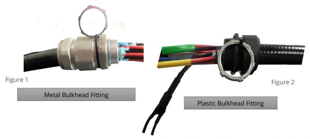
**Note:** If additional breakout length is needed, loosen the bulkhead and slide it down over jacket. Refer to the ripcord removal process in this document. Once the ripcord removal is completed, prep the end of the cable using a knife and remove 2.6 inches of the jacket to expose the outer copper armor.
