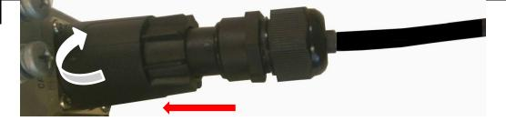
Slide the FullAXS compatible sleeve up to the RRH. Turn top nut clockwise to secure to RRH bulkhead connector.
