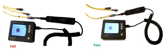
**Important Note:** In the event of failure, clean connectors as shown below, refer to optical fiber cleaning section within this document for additional cleaning suggestions.
