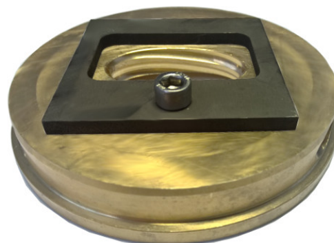
Picture shows flanging die for E65 waveguide
