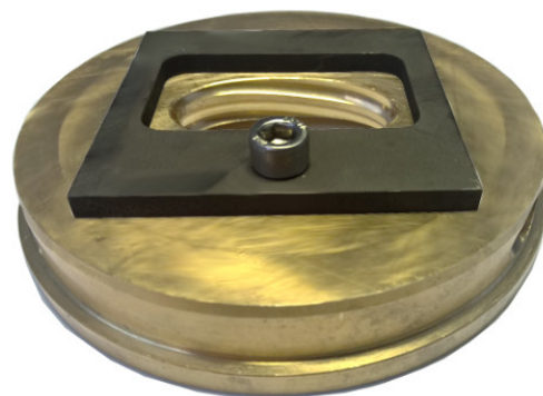
Picture shows flanging die for E65 waveguide
