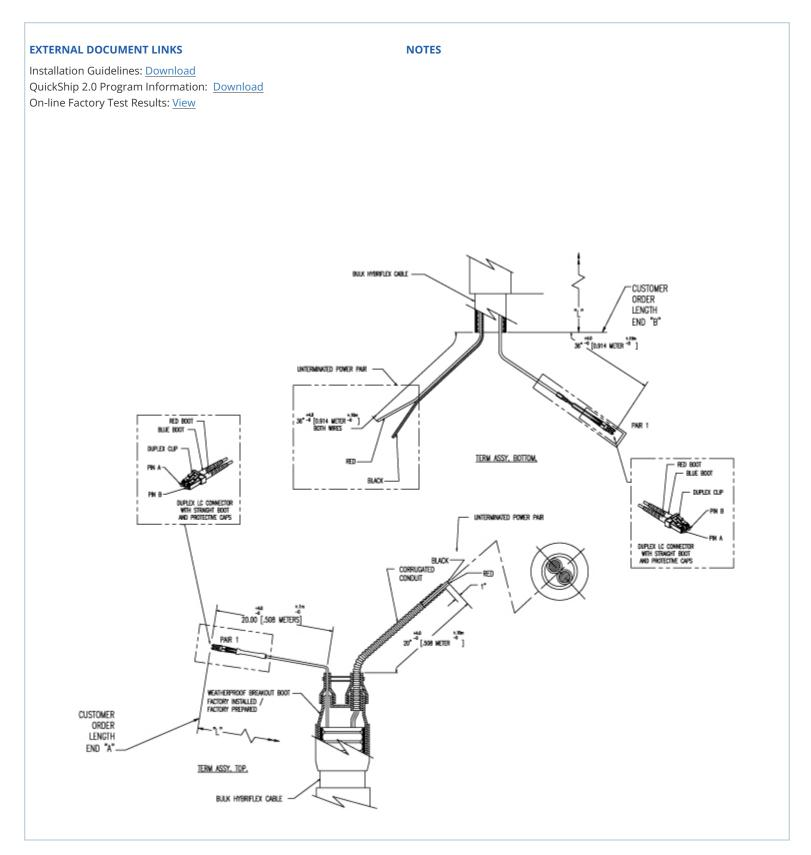
HYBRIFLEX® RRH Hybrid Jumper, 5/8", 1 pair 8AWG, 1 pair Single-Mode Fiber with DLC Connectors
