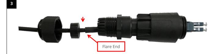
Wrap the rubber split grommet around the jacketing and VERY CAREFULLY push it UNDER the clamping fingers until the grommet is flush with the finger ends. Caution: it will be necessary to gently lift the fingers.
