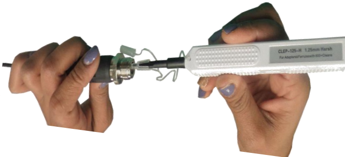
Cleaning ODC socket using the 1.25mm one-click cleaner
