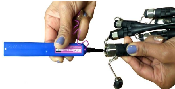
Cleaning ODC plug using the one-click cleaner
