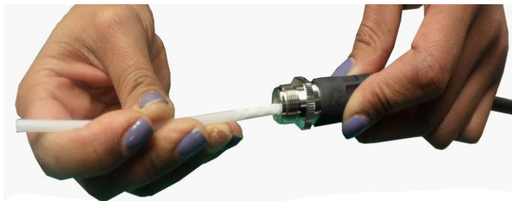
Cleaning ODC socket using the 1.25mm one-click cleaner
